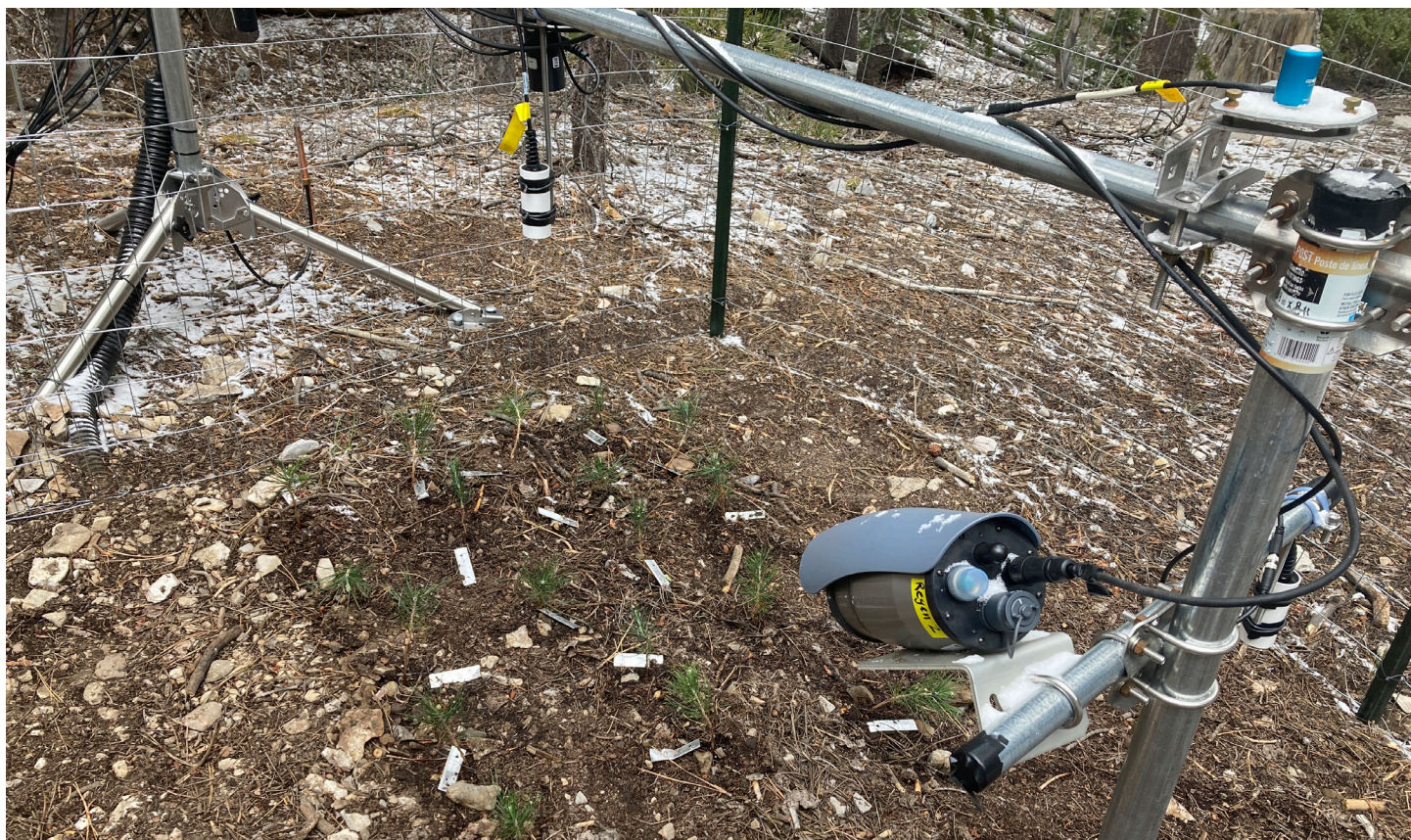
Photo of instrumentation used to monitor planted seedling survival at HTNF. This site is in Scout canyon, near the existing SNOTEL station.
